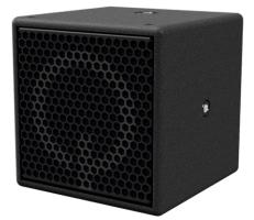
MODEL type filter power handling program power impedance sensitivity program SPL 1m peak SPL 1m frequency range dispersion weight size (wxhxd) C4 4"/1" coaxial 1-channel DSP control 100W 200W 8 Ohms 91dBWm 114dB 120dB 100Hz-18kHz 100<sup>e</sup> conical 2,5 kg / 5 lb 124 x 124 x 124mm 4.9 x 4.9 x 4.9 inch
