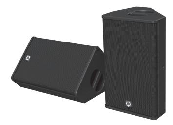
MODEL type filter power handling AES program power impedance sensitivity program SPL peak SPL frequency range dispersion weight size (wxhxd) U10 10"ND/1"ND universal full range system passive 500 W 1000 W 8 Ohms 97 dB 1W/1m 127 dB 1m 133 dB 1m 52-19 kHz 90°x40° hxv 16 kg 325 x 525 x 295 mm
